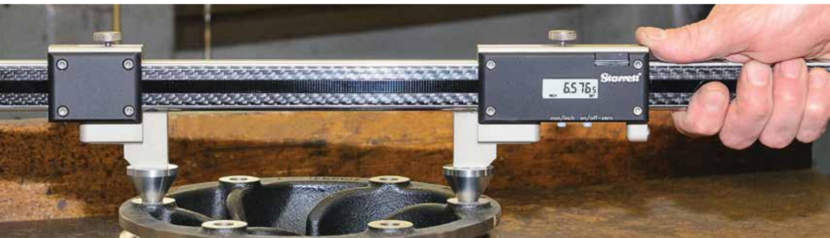
5002BZ-40/1000 with PT06137 Disc Contacts
