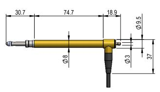
8 mm After Electrical Zero, Halfbridge, ±2 mm Measuring Stroke, Setting 1:2
