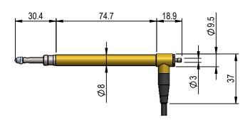
8 mm Stroke After Electrical Zero, Halfbridge, ±2 mm Measuring Stroke, Setting 1:1
